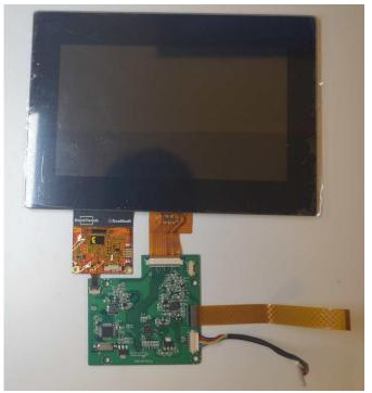
Plug in the USB bridge Cable on the 10 pin side on the DSI board
