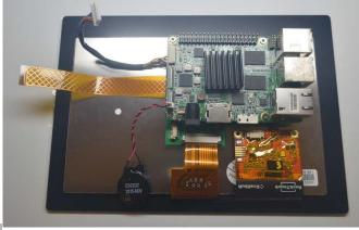
Now Plug In the USB Cable and the DSI Cable over the UP board connectors
