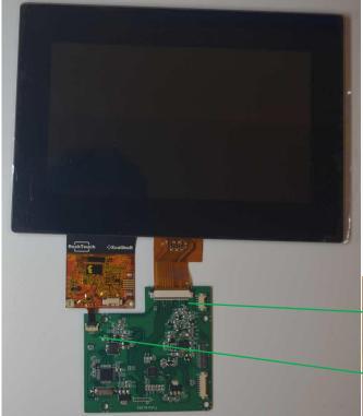
Plug in the 4 pins Touch FPC into the 4 pins ZIF connector and then plug in the 40 pins Display FPC into the ZIF connector on the DSI board, and lock the connectors gently, make sure the FPC are correctly aligned
