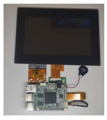
Now turn the display on the front side, and put back the board on the bottom. Connect the HDMI cable to an External LCD monitor and Plug in the power supply on the UP board
