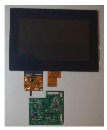
Bring the Display with touch and align n front of the DSI converter board, open the two ZIF connector on the DSI board
