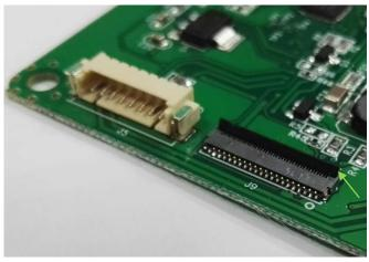
Open the DSI 41 Pin connector from the back side
