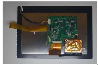
Bring the board on the Back side of the LCD, and fix the 4 spacer with the 4 nuts
